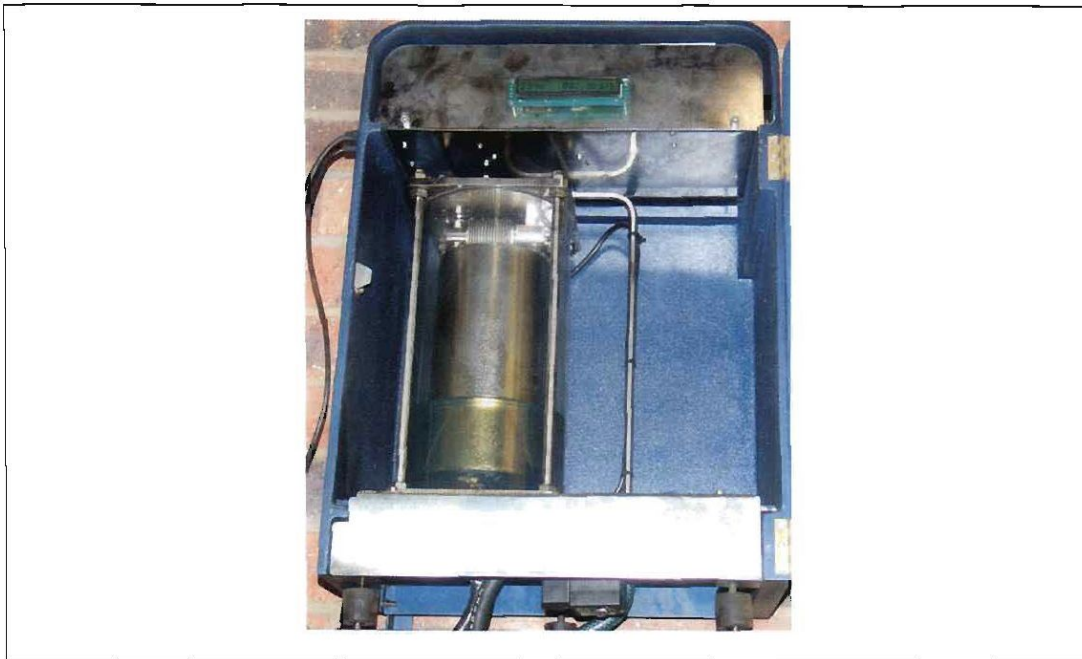
Figure 21: Gravity fuel flow meter
