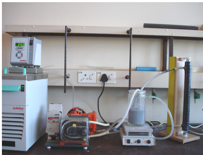
Figure 9 Photograph of the photocatalytic flow reactor system with temperature control unit and peristaltic pump
