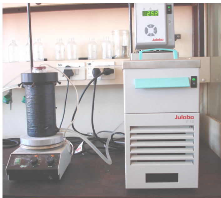
Figure 7 Photograph of the photocatalytic batch reactor system with connected recirculating temperature control unit
