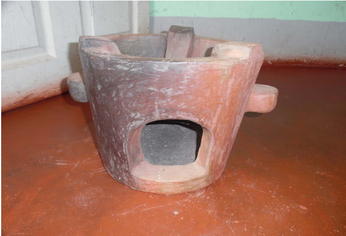
Image 4.11: An improved cooking stove (Tsotso stove) introduced to rural households in Chivi District
