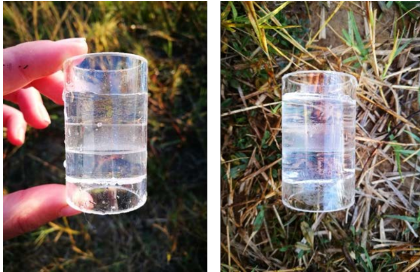
Figure 4-4: The artificial mussel design (Wu et al. , 2007).
