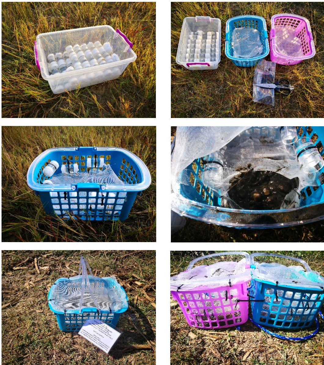
Figure 4-6: Steps taken to assemble the plastic baskets for the artificial mussels and transplanted clams.
