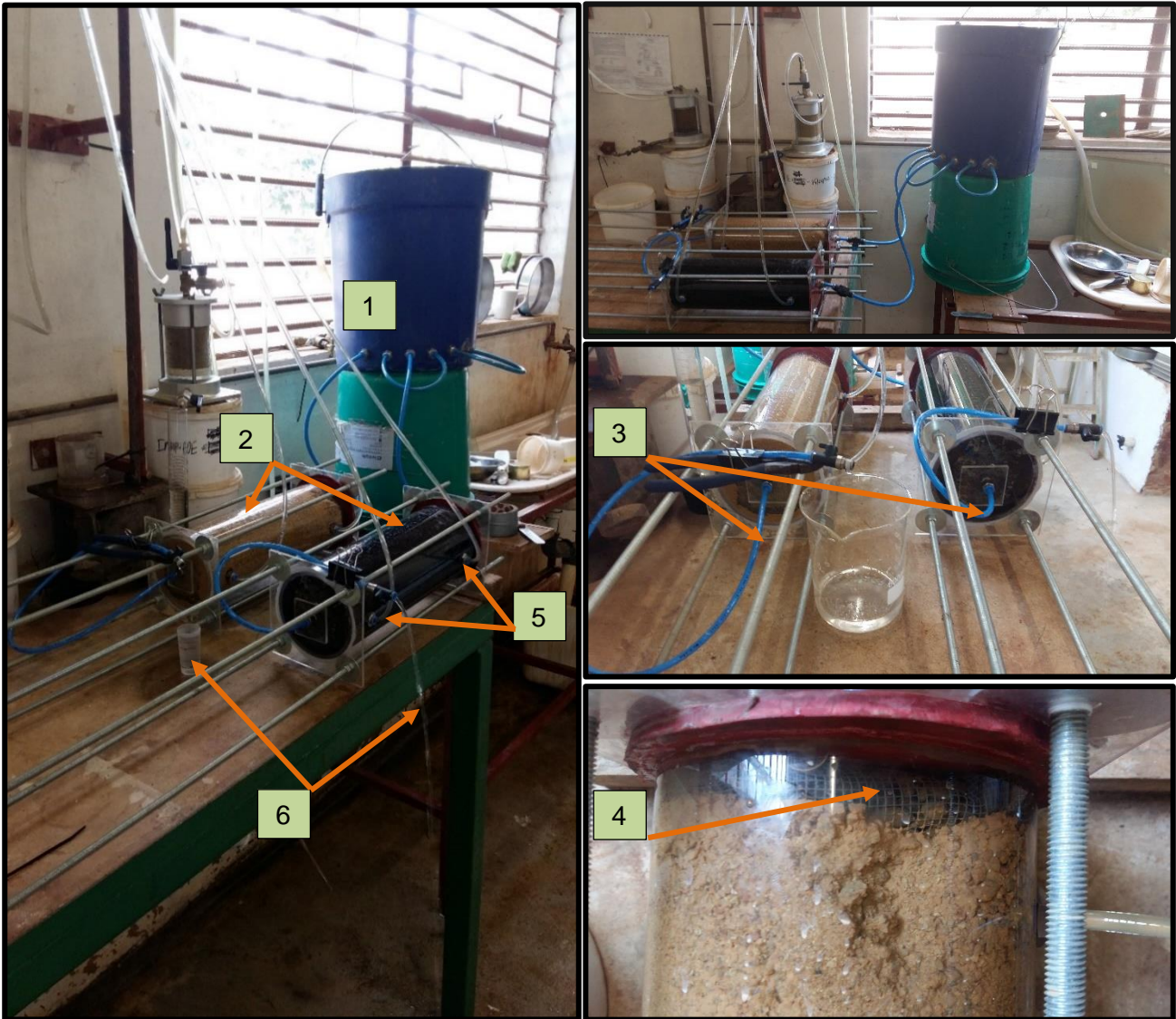
Figure 15: Experimental setup to assess hydraulic properties within each substrate mixture by means of a constant head permeability test.
