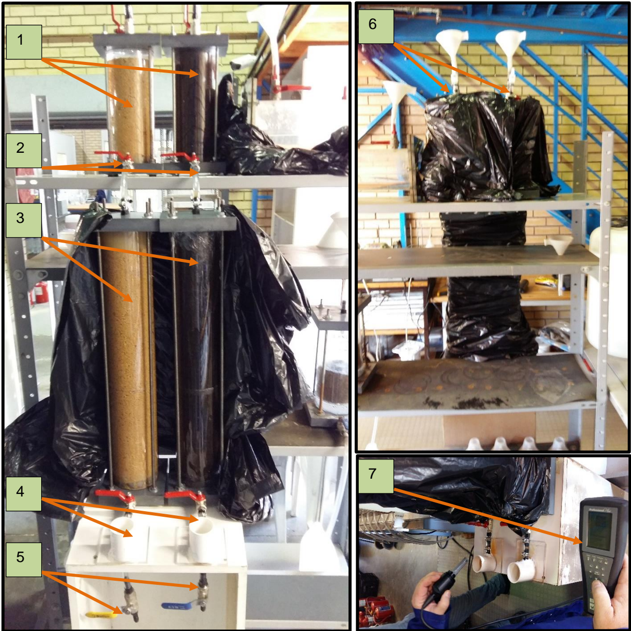
Figure 13: Experimental setup to track changes in dissolved organic carbon concentration over time.
