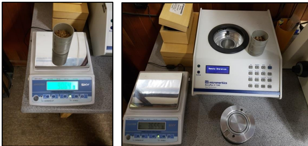
Figure 16: Sample measuring and Pycnometer to calculate relative density.
