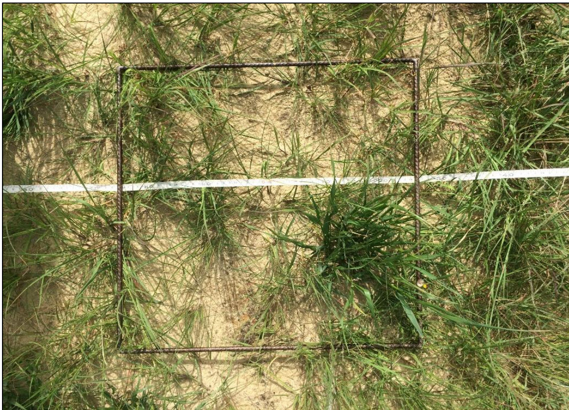
Figure 3.27: The 0,25 m 2 steel quadrant used on transect line to determine the density of the species at the Crown and Rooikraal gold TSF trial plots. Photo taken by C.A. Kruger, 15/11/2016.
