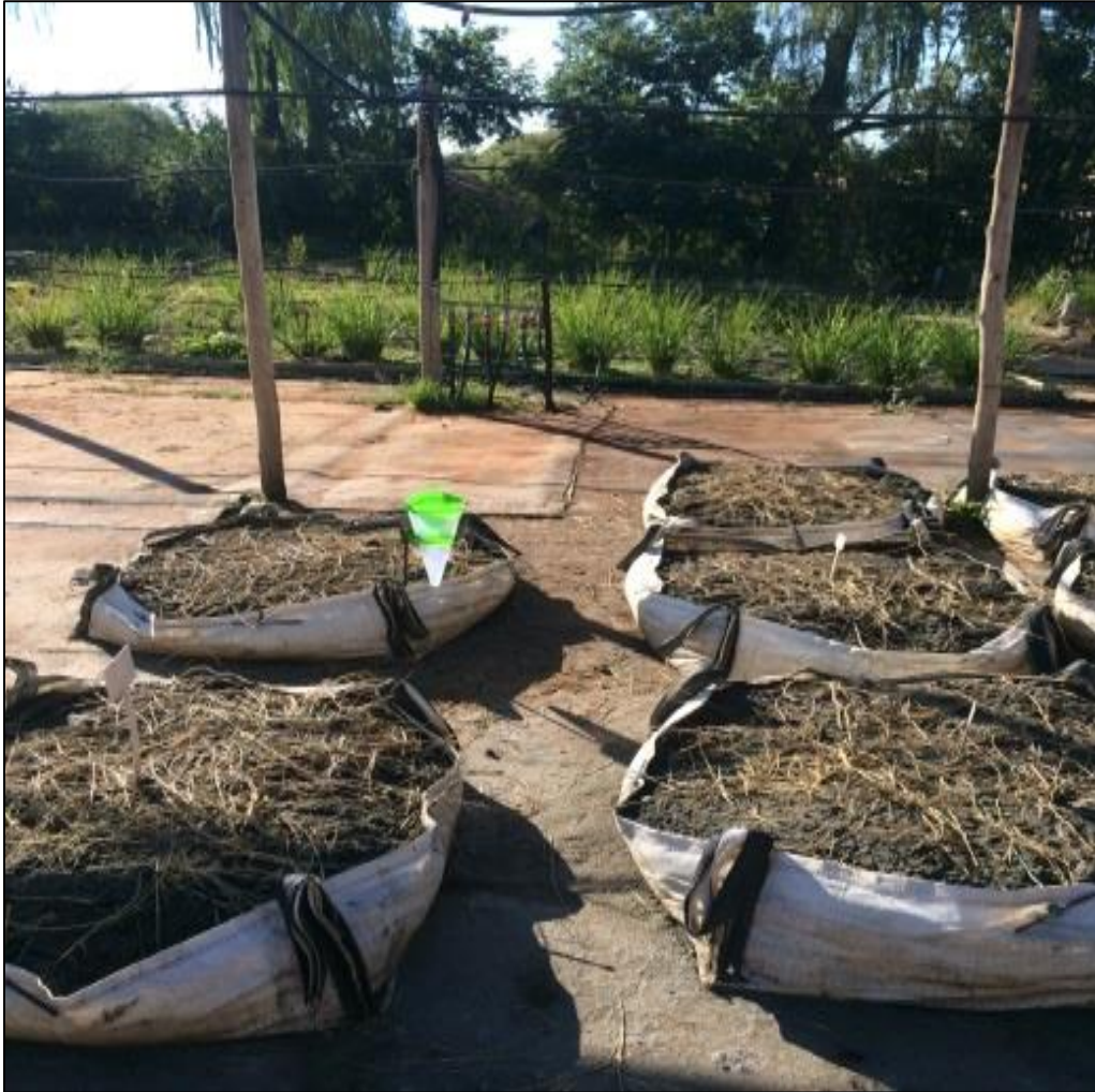
Figure 3.17: Platinum tailing material trials in bulk bags after amelioration, mulch application and sowing. Photo taken by C.A. Kruger, 4/6/2016.
