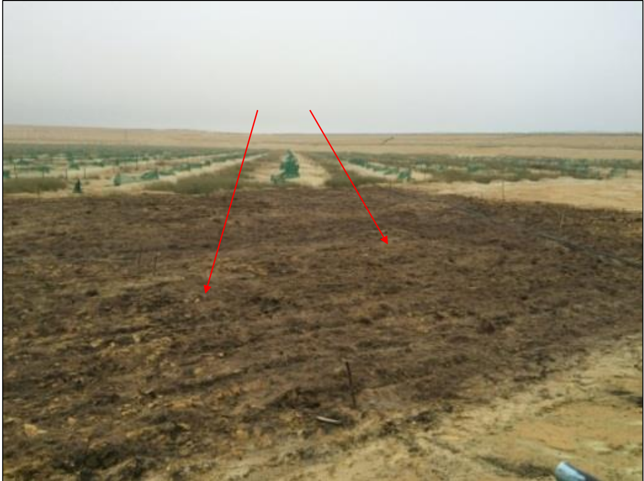
Figure 3.15: Trial plots at the Crown gold TSF site with mulch applied after amelioration and sowing. Mulch overlaying plots are indicated with red arrows. Photo taken by C.A. Kruger, 9/3/2016.
