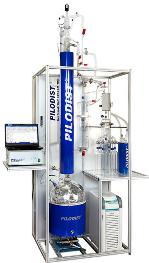
Figure 3.2. Pilodist 104 (PD104) distillation apparatus (Pilodist GmbH, n.d.).
