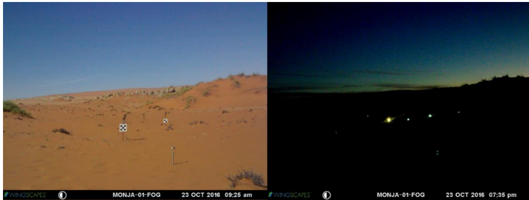
Figure 25: a) Photograph from Wingscape time-lapse camera with checkerboard markers set up at 10 m and 20 m distances from the camera to measure visibility during a daytime fog event and b) spotlights set up at various distances to determine the visibility during a night-time fog event
