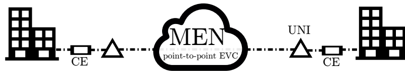
Figure 6: Example of ethernet line service
