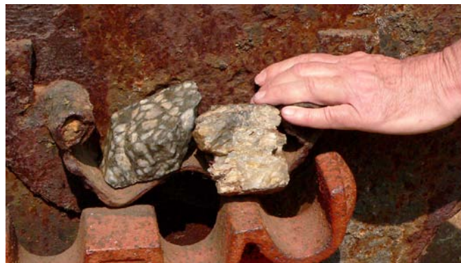
Figure 6.3: Examples of gold-bearing ores. Conglomerate (left) from a Witwatersrand Gold Mine and quartz vein (right), Old Kromdraai Visitor Mine
