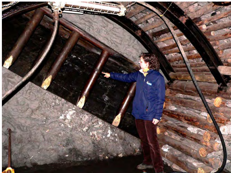
Figure 4.11: Coal seam stope, Visitor Coal Mine, Deutsches Bergbau-Museum (German Mining Museum), Bochum, Germany
