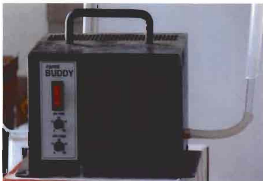
Figure 3.1: Sterizone Buddy ozone generator with a capacity to produce 300mg ozone/h. Mass= 3.9kg, Dimension= 109mmX180mmX150mm.
