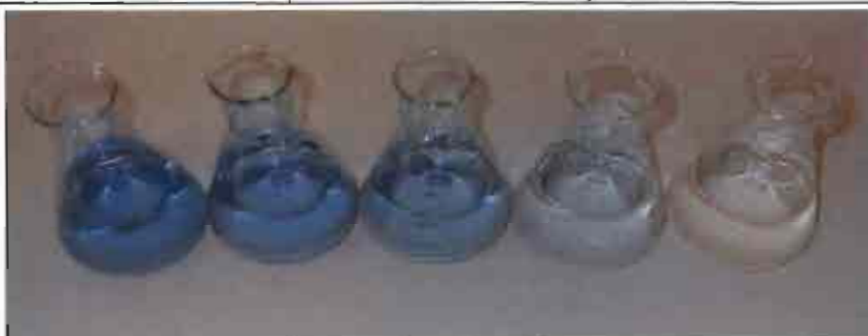
Figure 3.3: Photographs showing the effect of increasing ozone concentration on indigo dye. As the concentration of ozone increases in the flasks from left to right, the colour of the indigo decreases.
