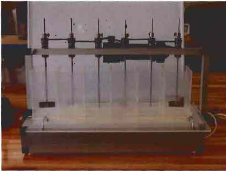
Figure 5.1: Jar Test Apparatus that was used in this study. It consists of 6 beakers, each with a capacity of 1 liter, with paddles and speed gauge.
