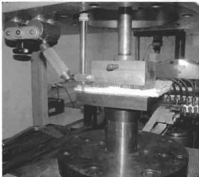
Figure A.1: The experimental set-up for measuring the compression behaviour of the different preforms.
