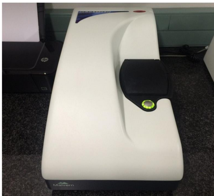
Figure C.4: The Malvern Zetasizer Nano ZS used to measure the zeta-potential, Pdl and size of the dispersions
