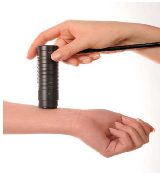
Figure E.3: Measurement with the Cutometer® MPA 580 (Adapted from Courage & Khazaka electronic GmbH, 2016c).
