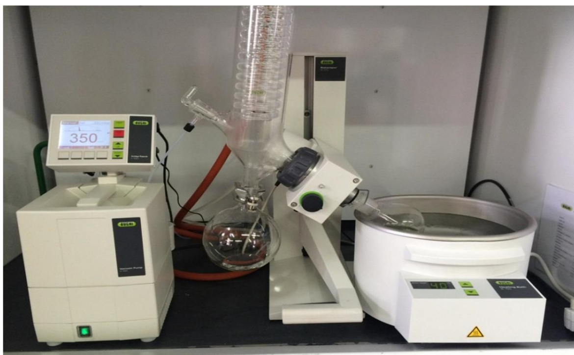
Figure B.1: A Büchi® (Switzerland) rotary evaporator equipped with an Interface I-100, Vacuum pump V-100, Rotavapor® R-100 and Heating bath B-100 was used during the formulation process
