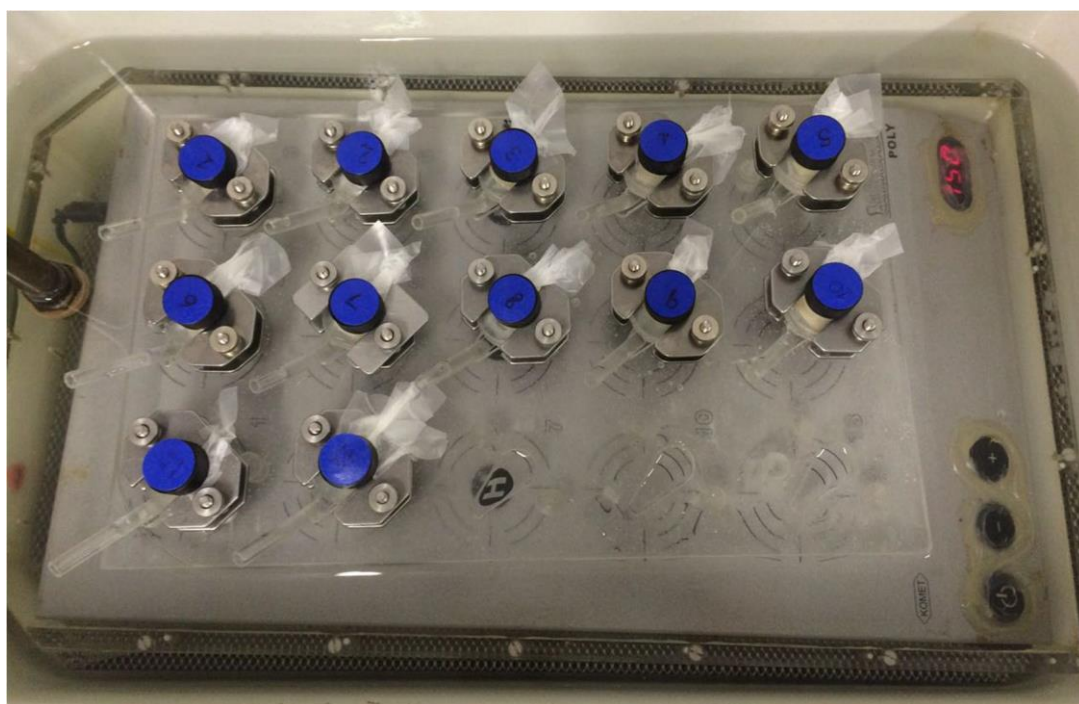
Figure D.3: Franz cells arranged on a Variomag® magnetic stirrer plate and submerged in a Grant water bath set at a controlled temperature of 37 °C
