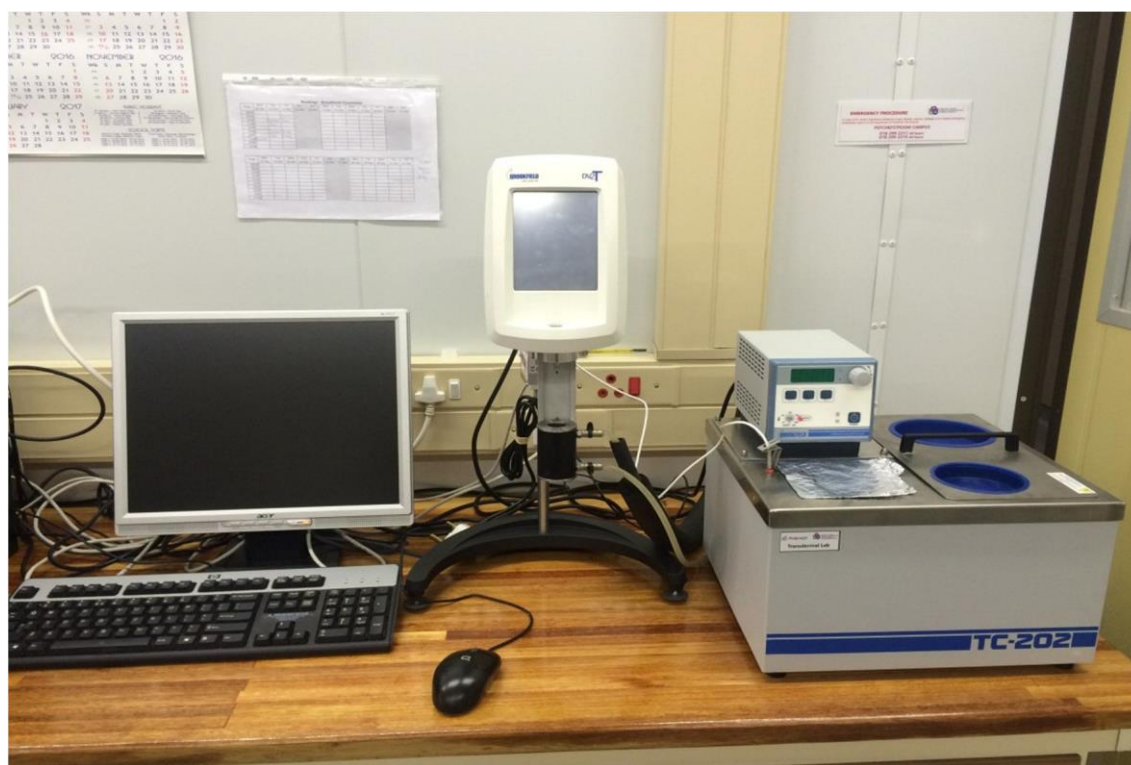
Figure C.2: Brookfield® Viscometer model DV III Ultra used during viscosity measurements
