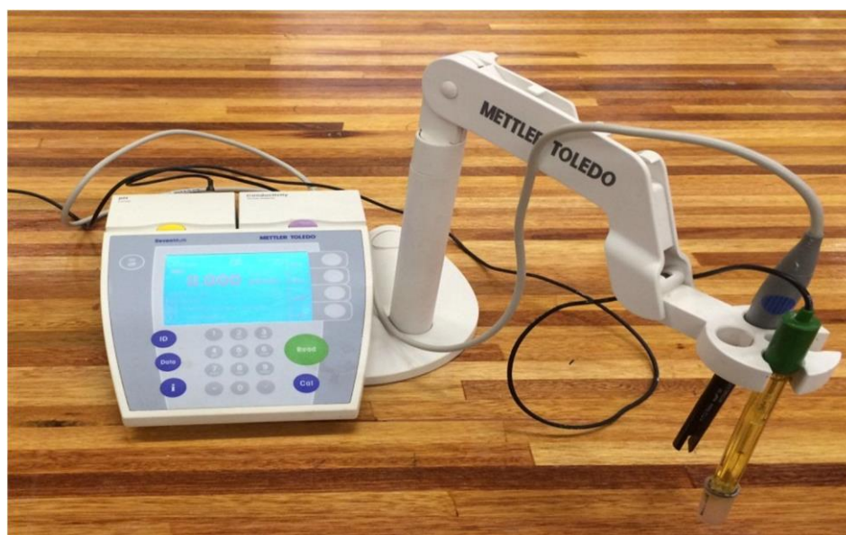
Figure C.3: The Mettler Toledo SevenMulti™ pH meter was used during the pH measurements, with a glass Mettler Toledo InLab® 410 electrode
