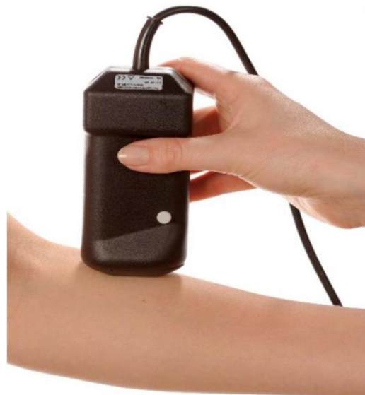
Figure E.2: Measurement with the Visioscan® VC 98 (Adapted from Courage & Khazaka electronic GmbH, 2016b).
