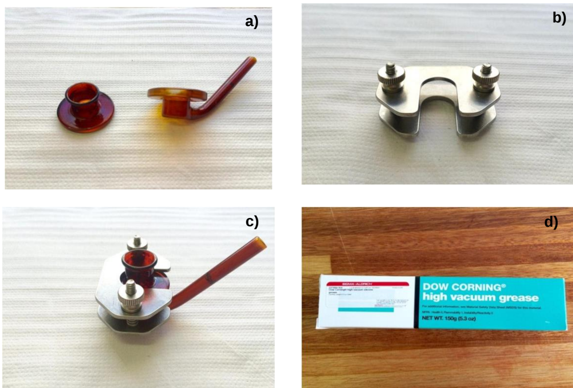
Figure D.2: Photographs illustrating a) the donor and receptor compartments of a vertical Franz cell, b) a horseshoe clamp used to, c) securely assemble the Franz cell and d) Dow Corning® high vacuum grease to prevent leakage
