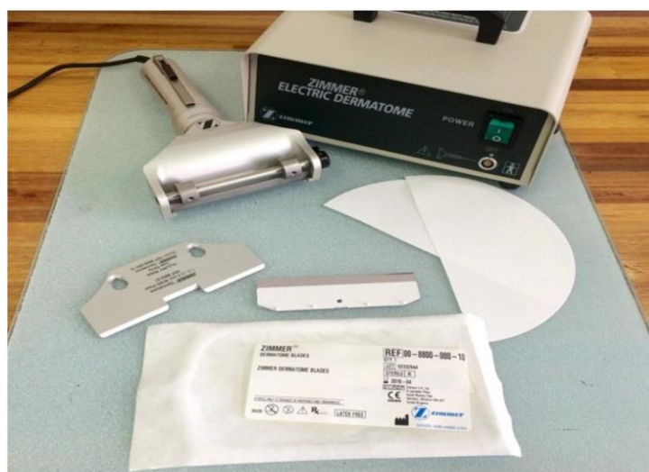
Figure D.1: The Zimmer™ electric dermatome with 2.5 cm width plate was used. Each donor's skin was dermatomed with a new sterile blade and placed on Whatman® filter paper
