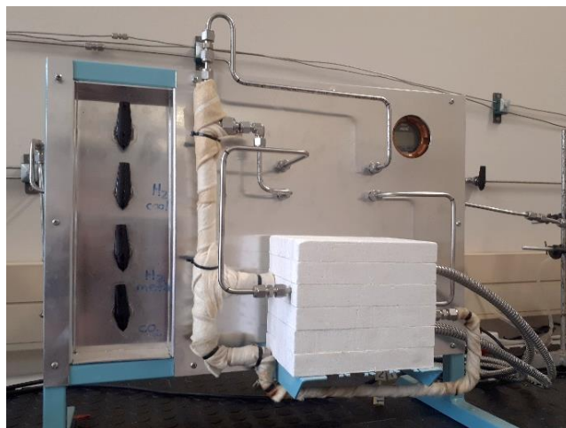
Figure 4.3: Sabatier reactor: surrounded by thermal insulation and with an external heat exchanger to pre-heat the cold methanation feed.
