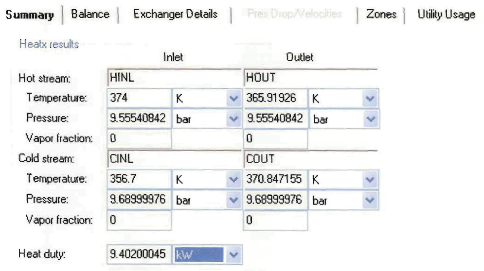
Figure E.3 – Desorber heat transfer validation
