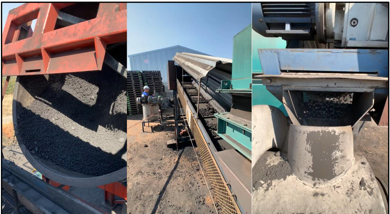
Figure 3-1: Production process of coal pellets, including drum pelletiser (left), conveyor system (middle), and rotary dryer (right) (provided by CoalTech™).
