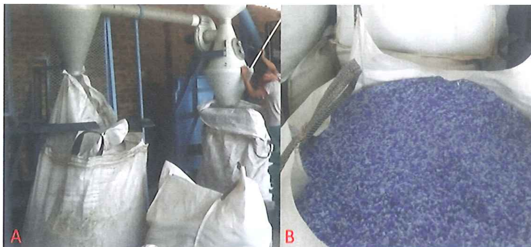
Figure 4.9: (A) Machine Used To Granulate Recyclables - HD. (B) By-products of Granulating Process.
