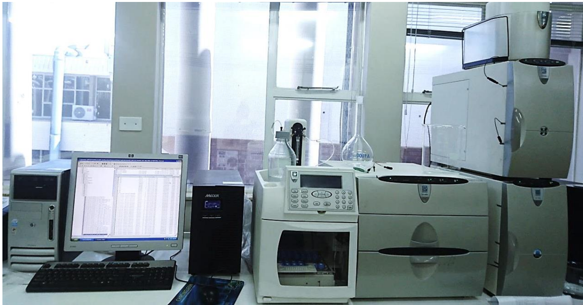
Figure 3.7 The Dionex ICS-3000 ion chromatographic system used for the ionic content analysis.
