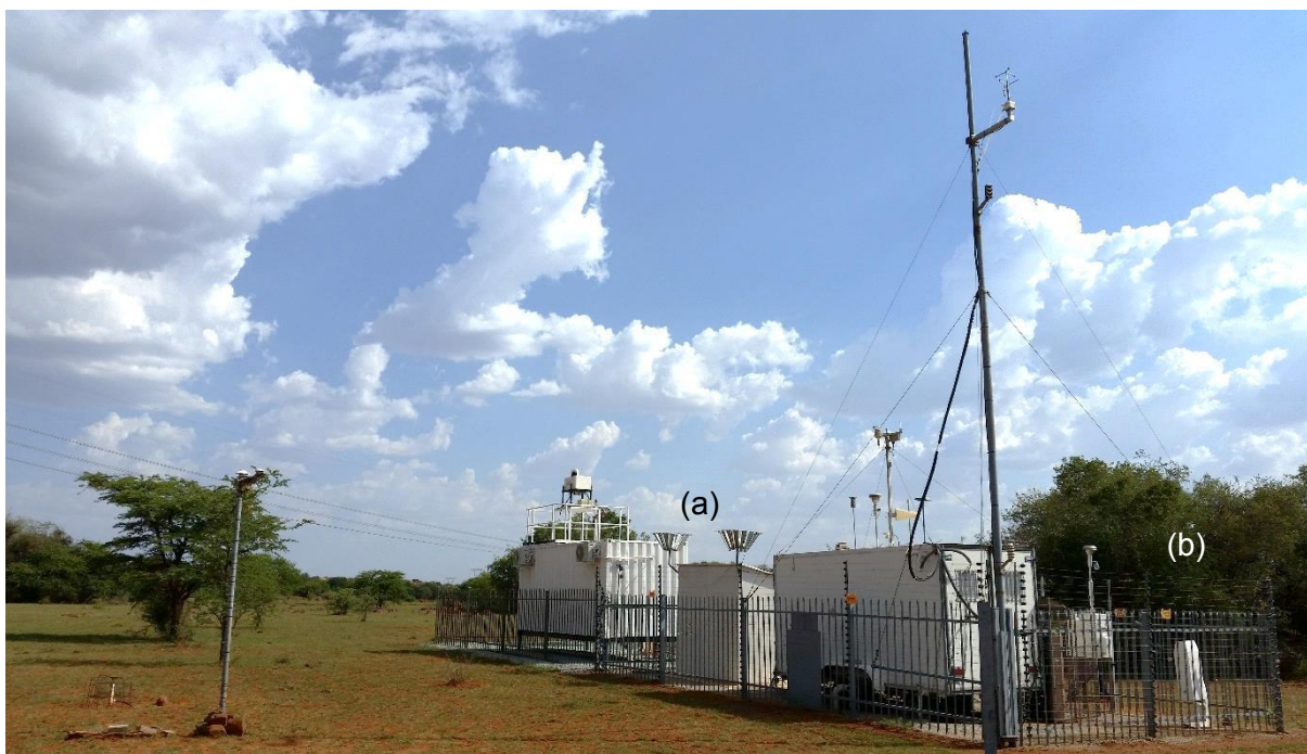
Figure 3.1 The Welgegund atmospheric measurement station with (a) the Vaisala and Casella rain intensity instruments indicated along with (b) the Vaisala CT25K ceilometer (Photo credit: Prof J.P. Beukes).
