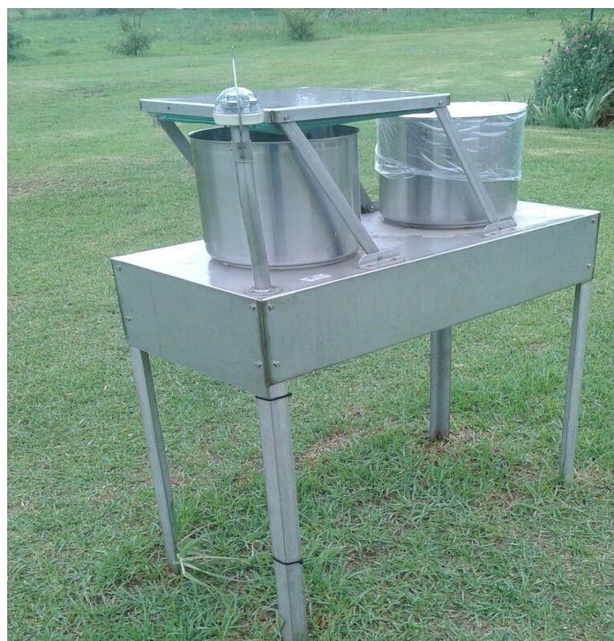
Figure 3.5: The wet-only sampler ( NWU Instrument Makers ). The open collection vessel is lined with a HDPE bag. The light-refracting sensor is visible at the foremost corner of the instrument. (Photo credit: Dr. M. Josipovic).
