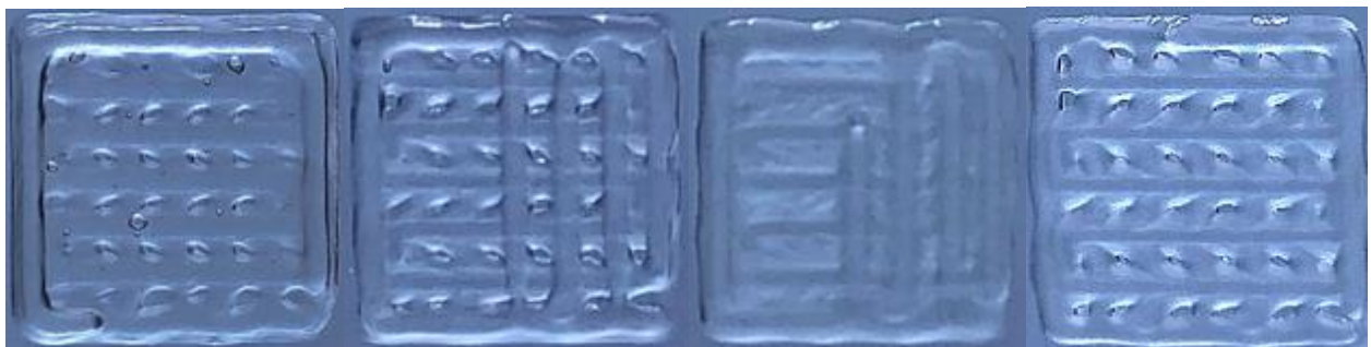
Figure 3-2: Photographs of 8 to 12% printed scaffolds of which the line width volumes exceed 8mm and 4mm expansion into each square within the design, on a 52mm extrapolation
