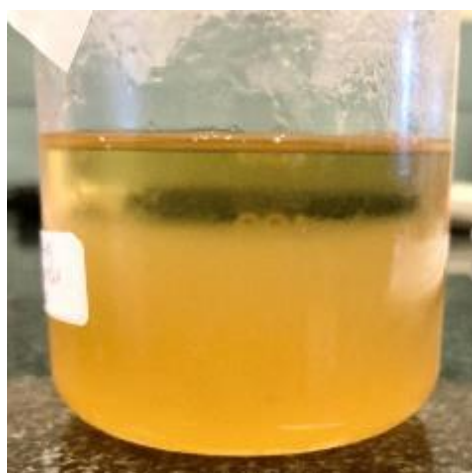
Figure A-1: Phase separation of alginate and PF127 as described in Table A-2
