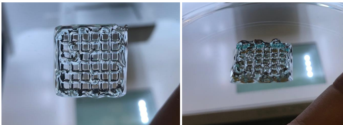
Figure 2-2: Four-layer printed grid scaffold using a sacrificial polypropylene oxide gel, Cellink® Start, top and side view of preselected CAD model, without optimised parameters
