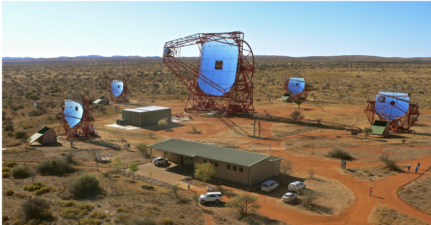
Figure 2.9: The H.E.S.S. site at the Goellschau farm. The five telescopes are visible: the four small telescopes H.E.S.S. I and the large telescope H.E.S.S. II at the centre ( https://en.wikipedia.org/wiki/File:H.E.S.S._II_gamma_ray_experiment_five_telescope_array.jpg ).
