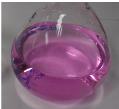
Figure 9.5 Photograph of the reducing substances impurity test solution on a commercially available sample of zinc acetate dihydrate.
