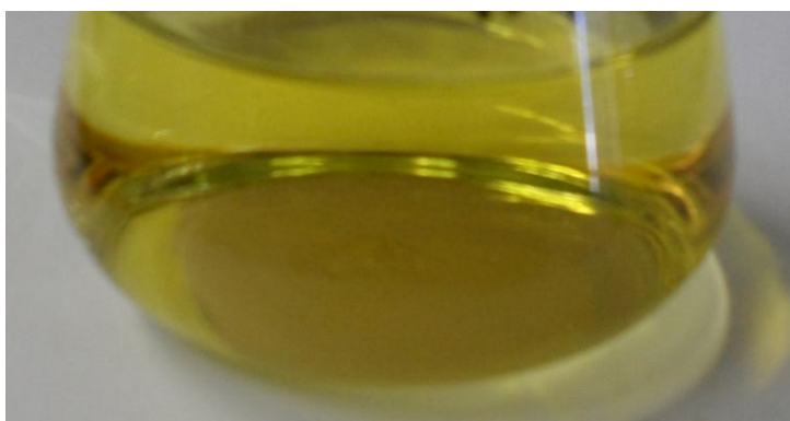
Figure 8.6 Photograph of the blank sample after the addition of the indicator and buffer agent.
