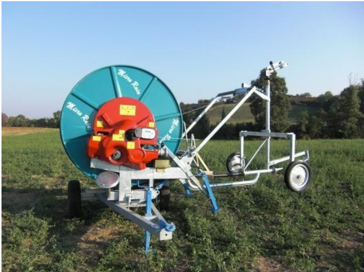
Figure 3. 4: OCMIS Traveller (Source: Irrigation Unlimited)
