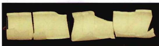
Figure 4.5: Warping and cracking of Alcoa casts after sintering
