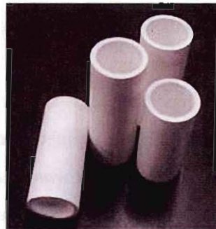
Figure 2.10: Tubular ceramic support made from Al_2O_3
