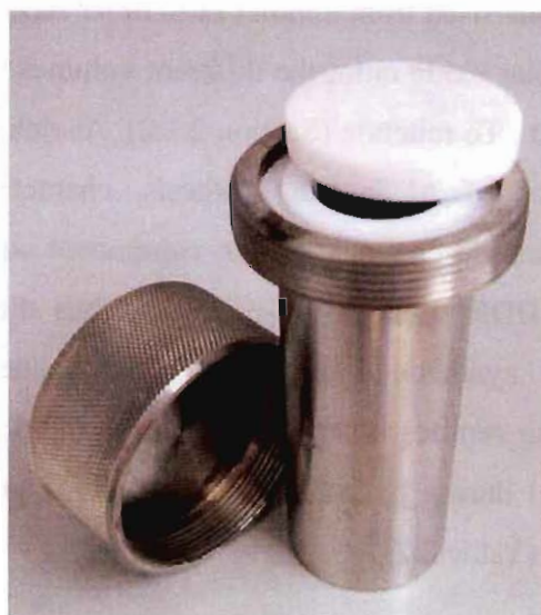
Figure 2.11: An example of a stainless steel autoclave with a Teflon insert
