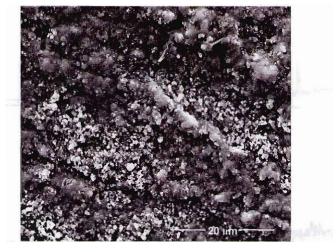
Figure 4.16: SEM showing the effect of zeolite adhesion after hydrothermal synthesis on an untreated ceramic support
