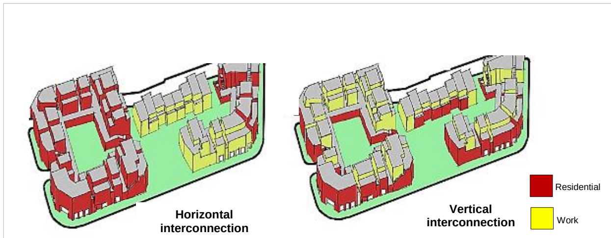
Figure 5-2: Illustration of horizontal and vertical interconnection of a multi-functional space. Source: Adapted from Placemakers.com (2013).
