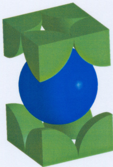
Figure 5-4: The body-centered tetragonal structure
