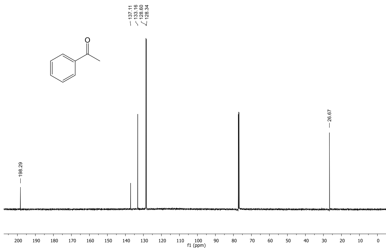
Figure S.8: ^{13}\text{C} \{^1\text{H}\} NMR (151 MHz, \text{CDCl}_3 ) spectrum of acetophenone.
