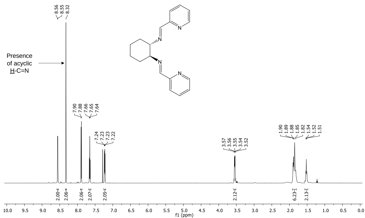
Figure 3.3: ^1\text{H} NMR (600 MHz, \text{CDCl}_3 ) spectrum of ligand S,S-L1.
