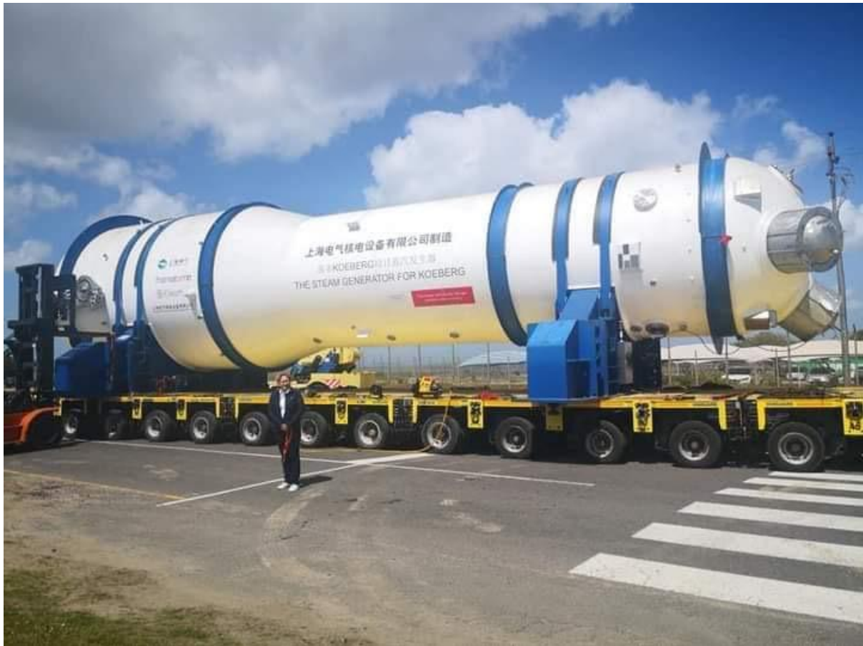
Figure 3-8: The first of the six Koeberg steam generators in Cape Town
