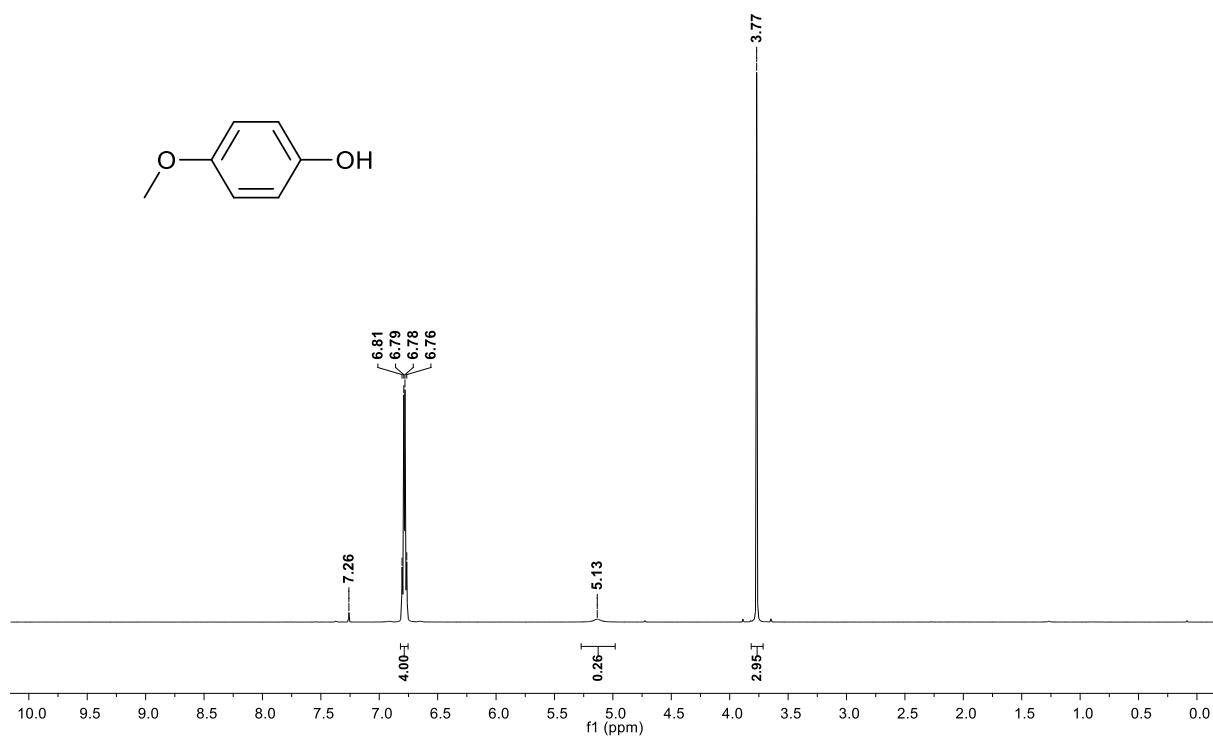
Figure S3.22: 1 H NMR (600 MHz, CDCl 3 ) spectrum for the hydroxylation of 4-iodoanisole to afford p -methoxyphenol (mequinol) as product.
