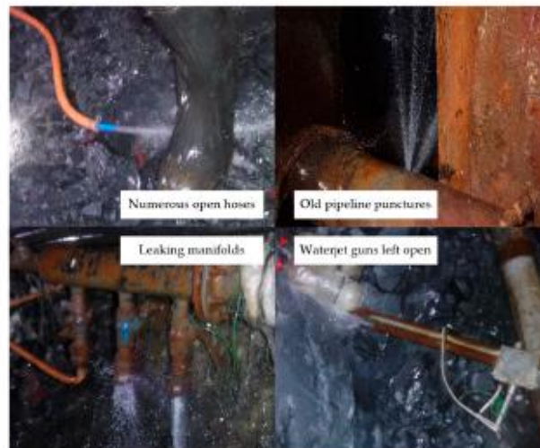
Figure 11. Common underground inefficiencies identified at case study mine captured by authors.
