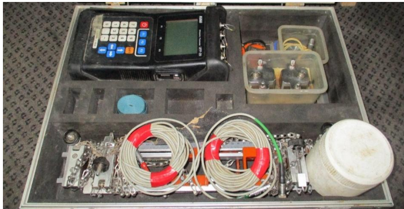
Figure 28: Ultrasonic water flow meter used.
