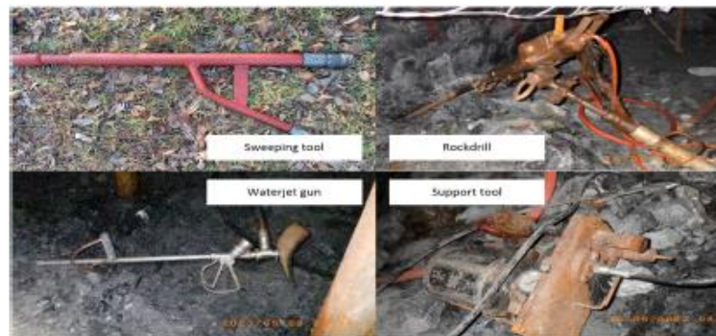
Figure 8. Water-consuming equipment at case study mine captured by authors.
