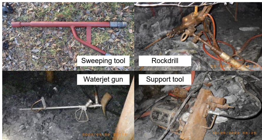
Figure 30: Intermittent water-consuming tools identified on Mine A.
