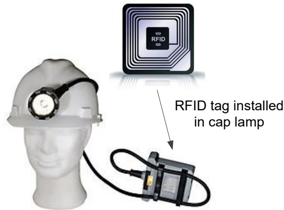
Figure 13: Example of RFID tag installed in cap lamps 1 2 .
