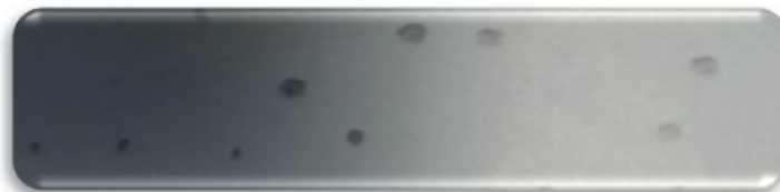
Figure E-7: Pinholes looks like small chips in the paint. (Duffy, 2004)
