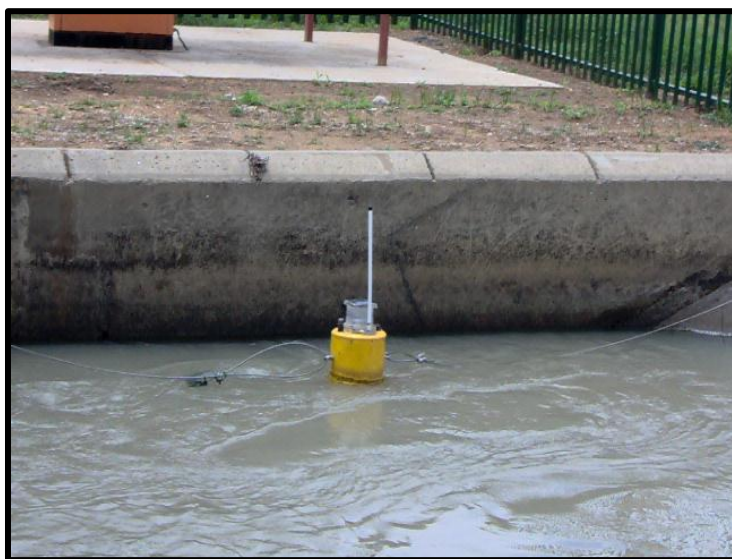
Figure 3.4 On-line ( in situ ) YSI 6600 V2 Multi-parameter water quality sonde in the canal measuring water temperature (°C), turbidity (NTU), conductivity (mS/m), dissolved oxygen (mg/L and % saturation), pH, chlorophyll- a (µg/L) and cyanobacterial cell concentration (cells/mL).
