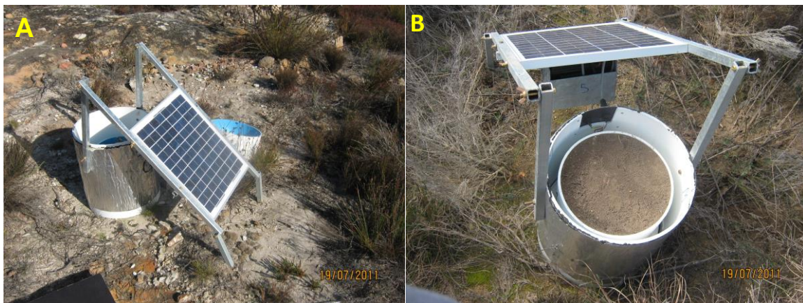
Figure 2.2. (A) and (B) Portable lysimeter comprising plain fynbos topsoil in a measuring pan.
