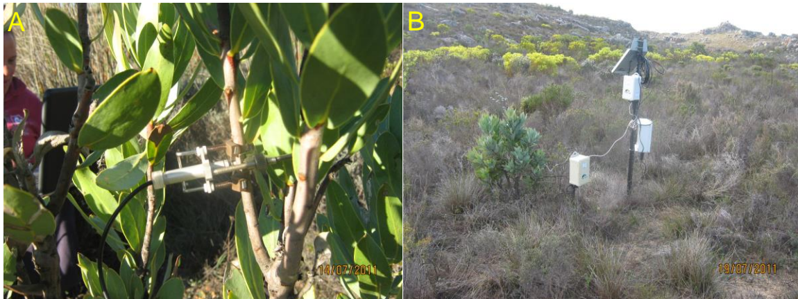
Figure 2.3. (A) and (B) Stem diameter sensor connected to plant.
