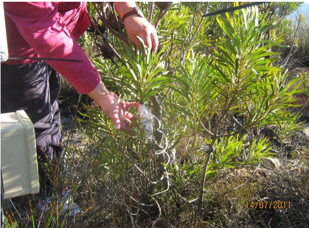
Figure 2.4. Sap flow sensor attached to the plant.
