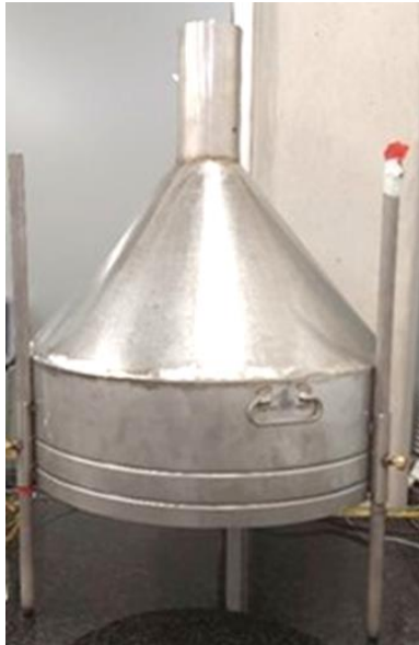
Figure 3-8. The emission capture hood.
