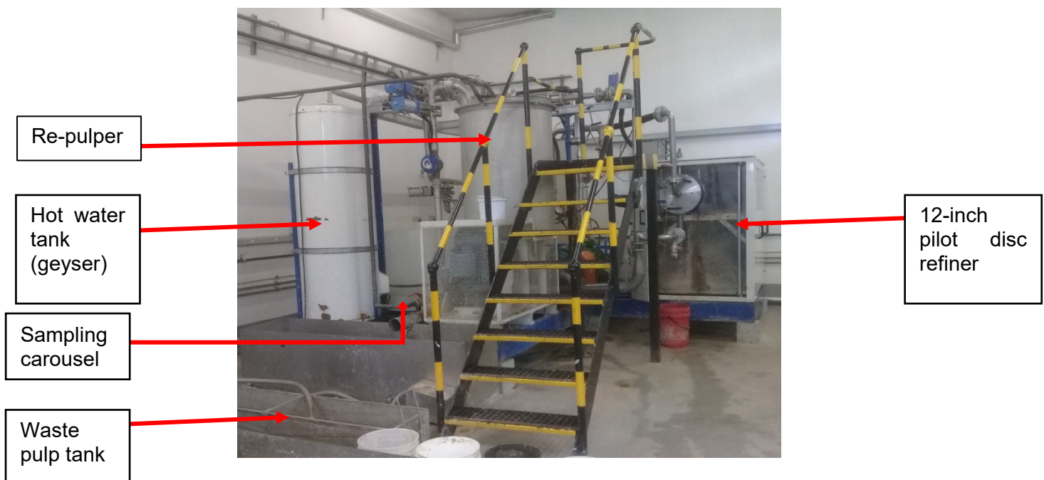
Figure 3-1: Image of the pilot refiner unit at the Sappi Technology Centre. The pilot refining unit comprises of a geyser, pump, sampling carousel, re-pulper with an impeller at the bottom, 12" single-disc refiner with a stator and rotor plates, a waste pulp tank, and an electrical switchboard.
