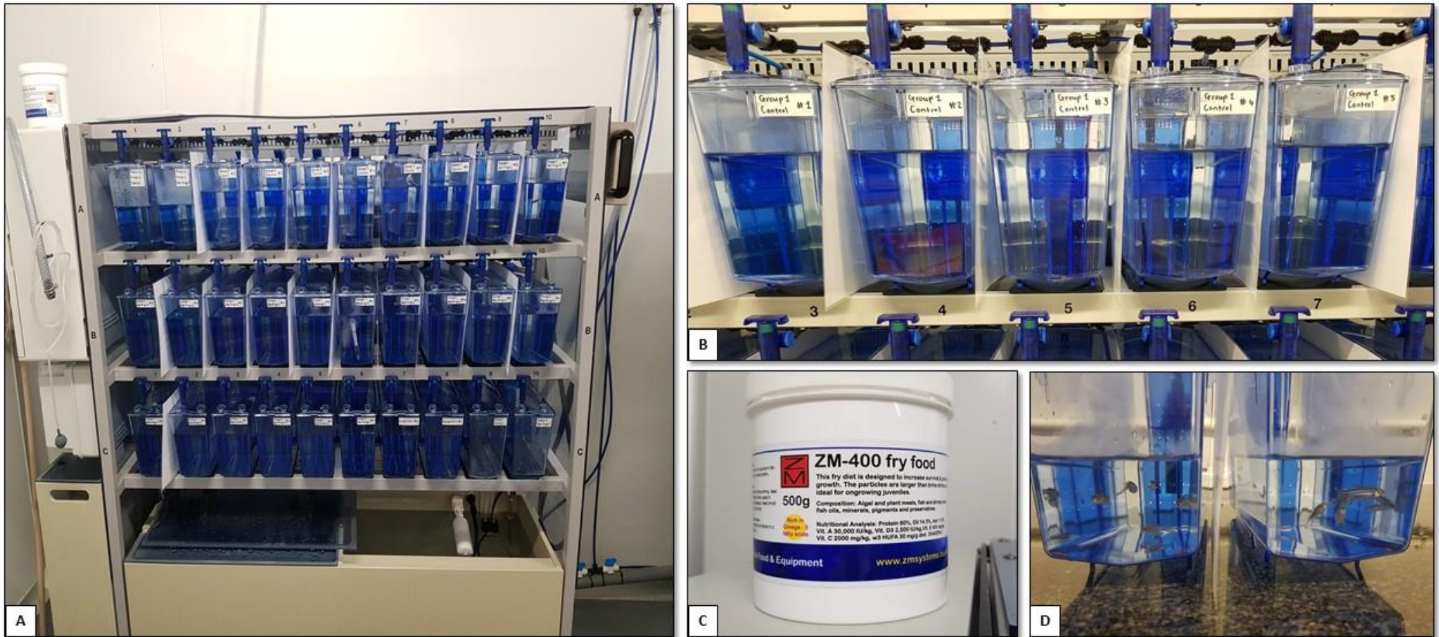
Figure D1 – ZebTec® Zebrafish Housing System (housed zebrafish according to standard laboratory conditions). B) Zebrafish acrylic tanks in the ZebTec® Housing System. Each tank was marked according to the group and fish number so that individual fish could be identified. White separators were placed between tanks to occlude the view of zebrafish in the adjacent tanks. C) Food provided to zebrafish throughout the investigation (ZM-400 fry food). D) Group exposure in tanks identical to home tanks. White separators were placed between the two tanks to occlude the view of fish from adjacent tanks.
