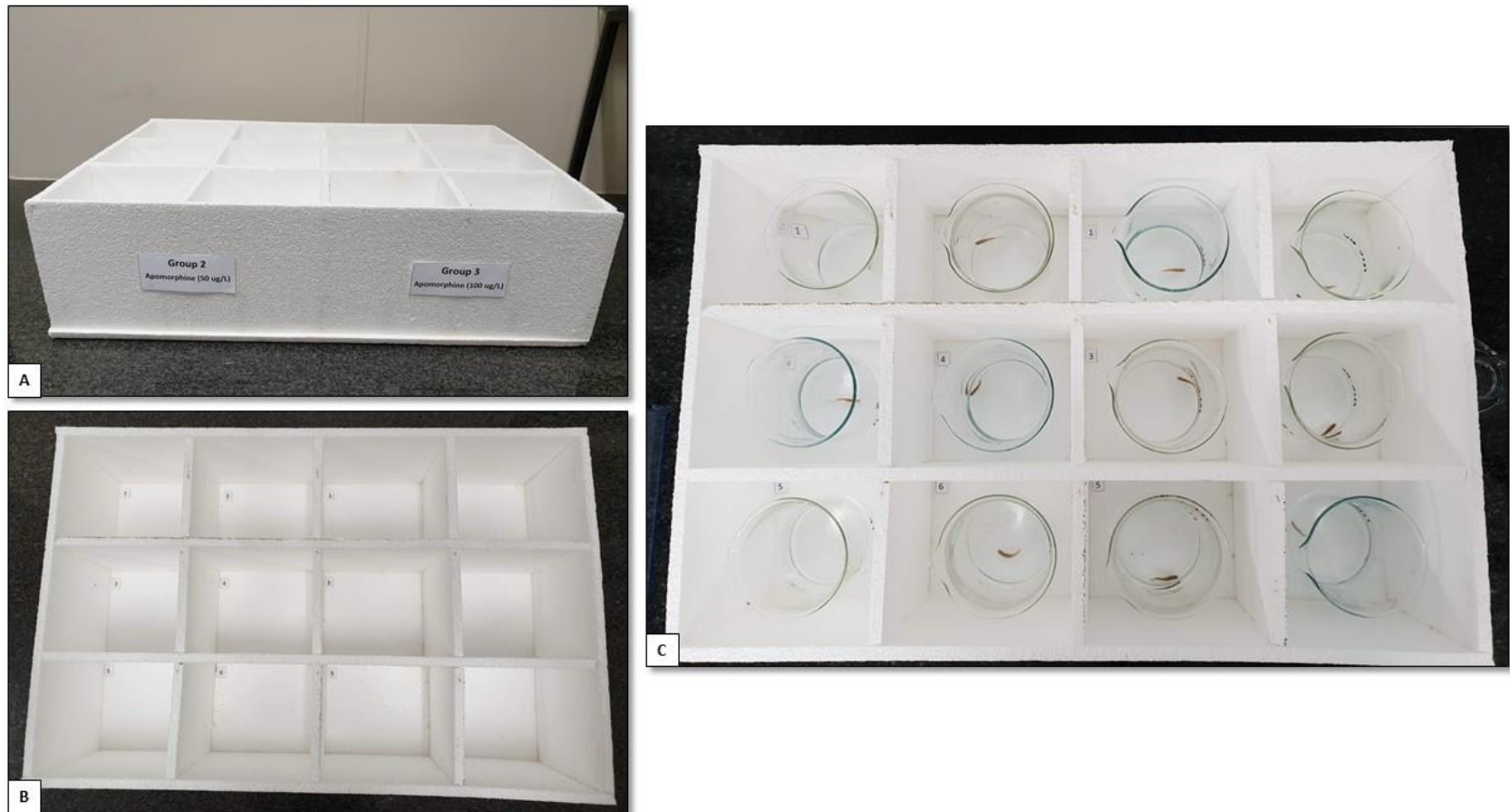
Figure D3 – A) Side view of polystyrene box used for individual drug exposure. Individually exposed groups ( n = 6 per group) could be identified by a label on the front of the box. Each compartment (6 on the left and 6 on the right) were also labelled individually from 1 - 6 to allow easy identification of zebrafish. B) Top view of polystyrene box used for individual drug exposure (12 compartments allowing for 2 groups of fish ( n = 6 per group) to be individually exposed simultaneously). C) Zebrafish exposed individually in 600 ml beakers that were placed in their individual compartments in the polystyrene box. Each beaker was numbered from 1 – 6 according to the number allocated to each individual zebrafish in their respective groups (as labeled on the home tanks) in order to ensure that each fish could be correctly identified and prevent confusion
