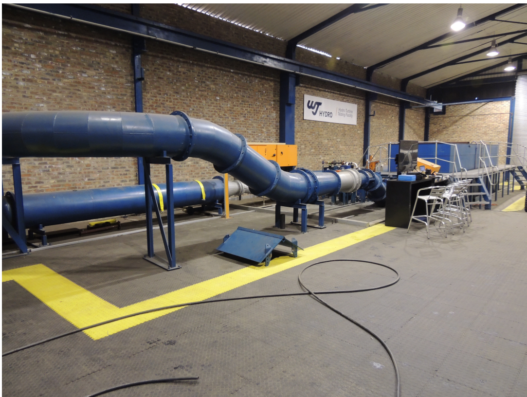
Figure 1.7. WJ Hydro Test Facility: outflow pipe from high pressure water tank, turbine housing and data logging system
