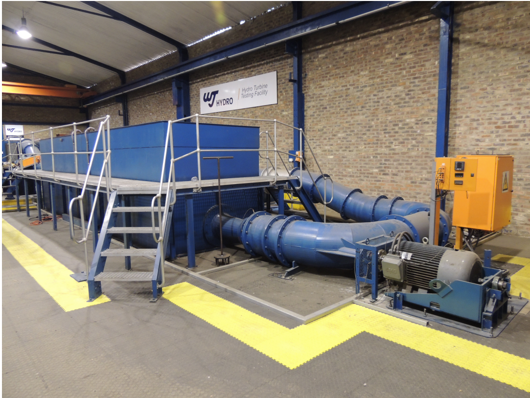
Figure 1.6. WJ Hydro Test Facility: axial pump, VFD and low pressure water tank
