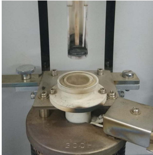
Figure 3.5: Image of the sample container of the TMA with the TMA furnace below it.
