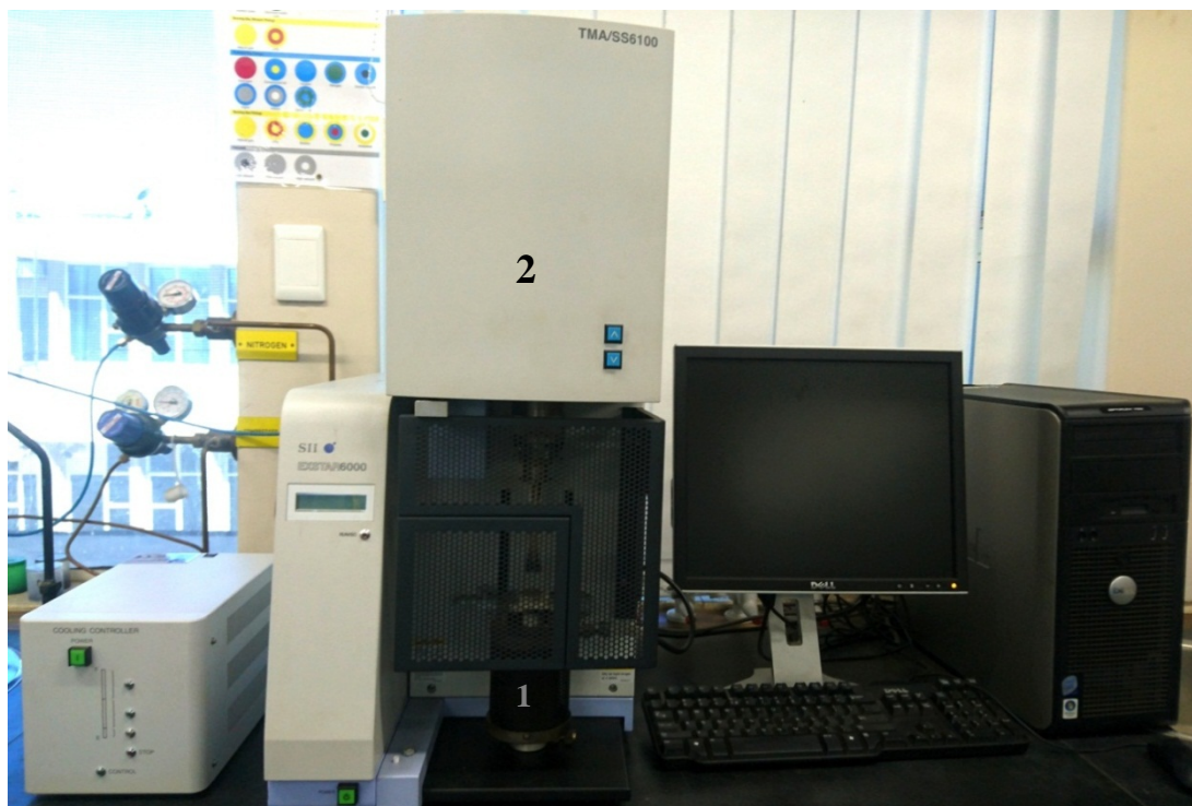
Figure 3.4: Image of the TMA instrument used with the section marked “1” being the furnace and “2” being the chamber.
