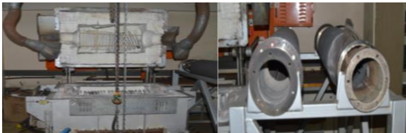
Figure 4.1: Open furnace showing heating elements (left), two kilns used for the ashing test with open front and back end (right)
