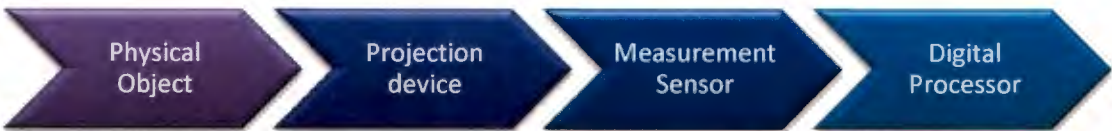
FIGURE 32: THE PROCESS OF DIGITISING COORDINATES WITH A NON-CONTACT DIGITISERS
