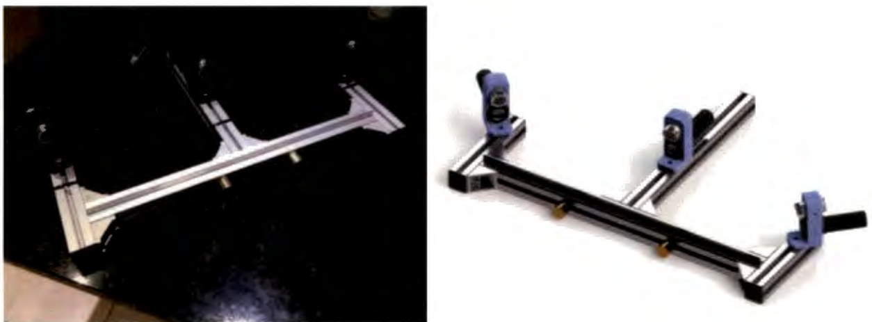
FIGURE 125: THE PROFILER THAT WAS DEVELOPED (LEFT) AND THE PROFILER THAT WAS DESIGNED (RIGHT)
