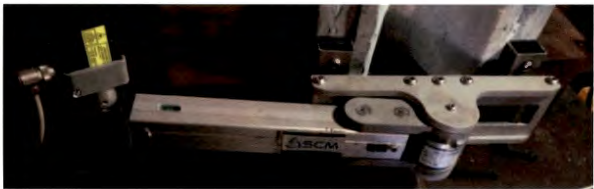
FIGURE 23: THE LASER BASED SHEAVE WHEEL PROFILER
