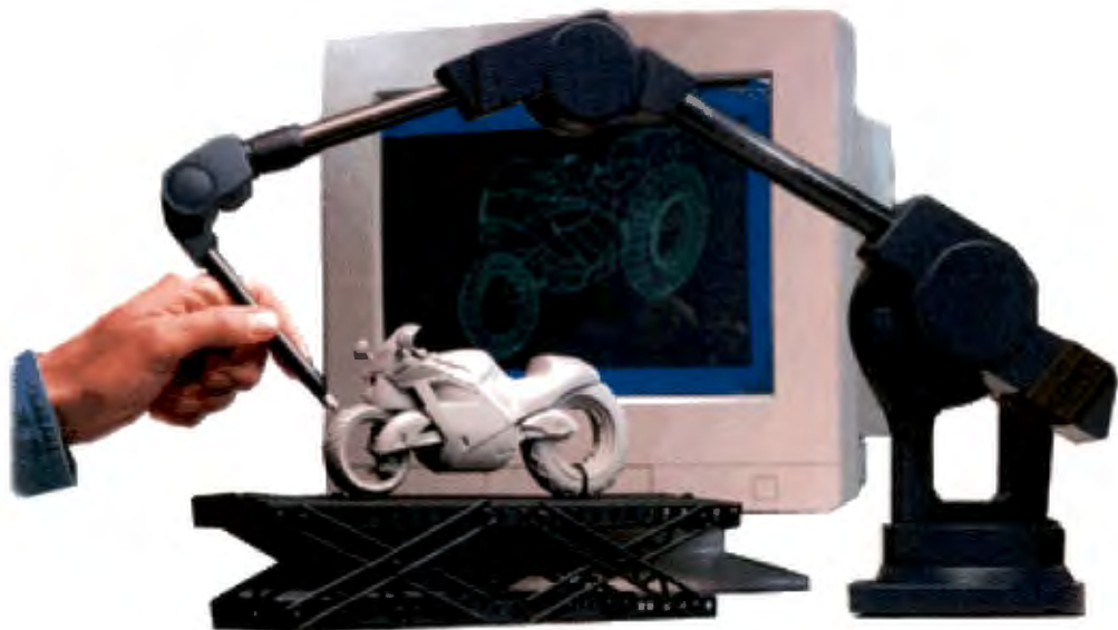
FIGURE 22: MICROSCRIBE COORDINATE MEASURING MACHINE
