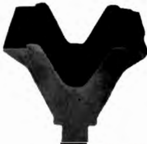
FIGURE 90: SHEAVE WHEEL SAMPLE THAT WILL BE PROFILED FOR SWE
