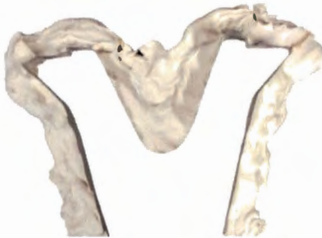
FIGURE 98: SHEAVE WHEEL PROFILE PLASTER CAST
