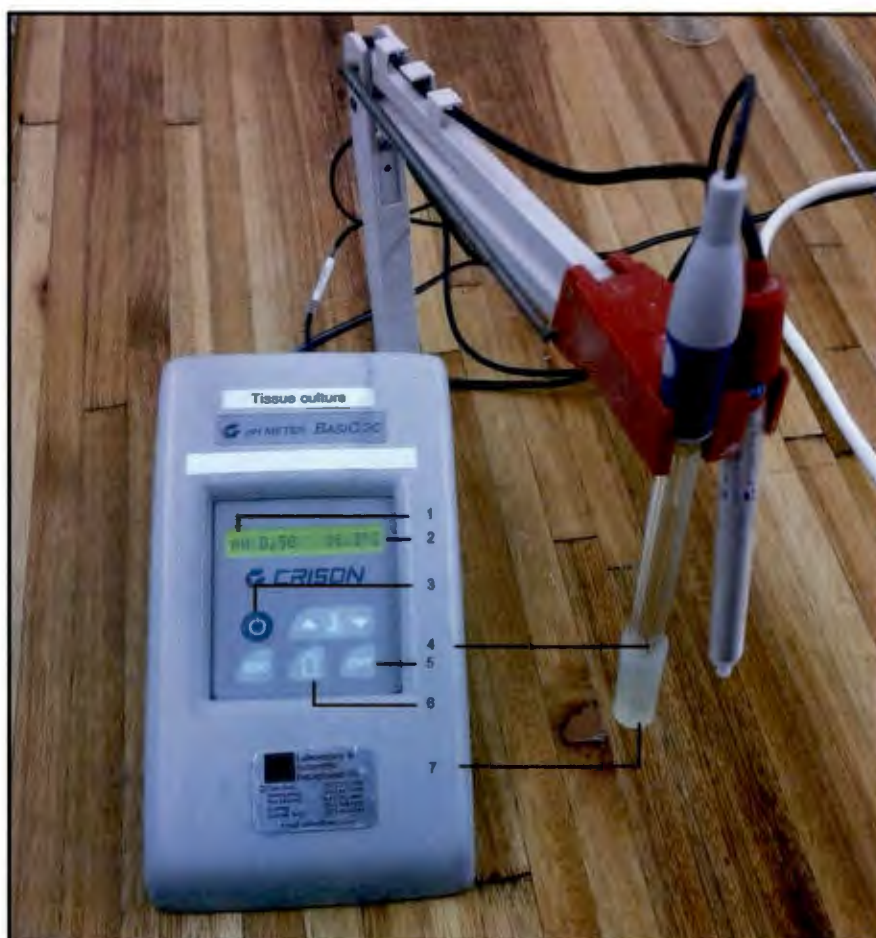
Figure 2.13: pH Reader (1-pH reading; 2-temperature reading; 3-on/off; 4-probe; 5-enter; 6-calibrate; 7-cap with salt water to protect probe)
