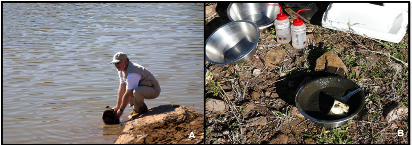
Figure 8: (A) Sediment sampled with a metal spade or cup and (B) mixed in pre-cleaned stainless steel containers to ensure homogenous samples.
