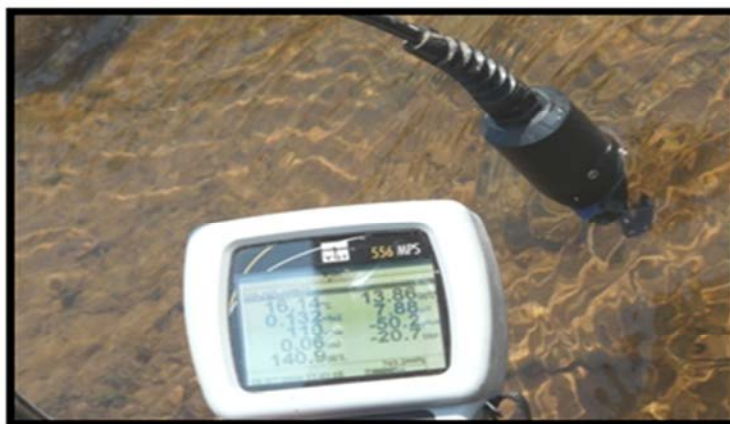
Figure 9: The in situ water quality of the different sites was measured using a handheld multi-probe meter.
