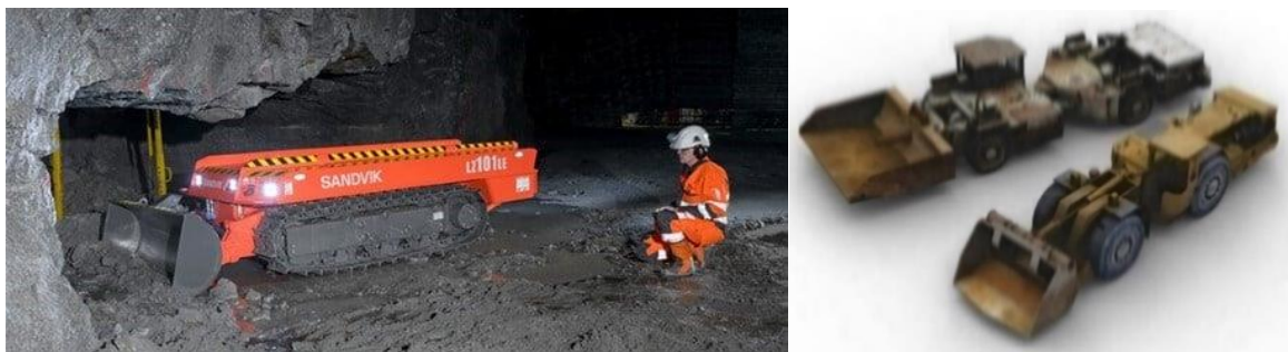
Figure 2.17: Examples of mining equipment that could be converted make use of the LOHC technology (left, XLP dozer; right, LHD machine).
