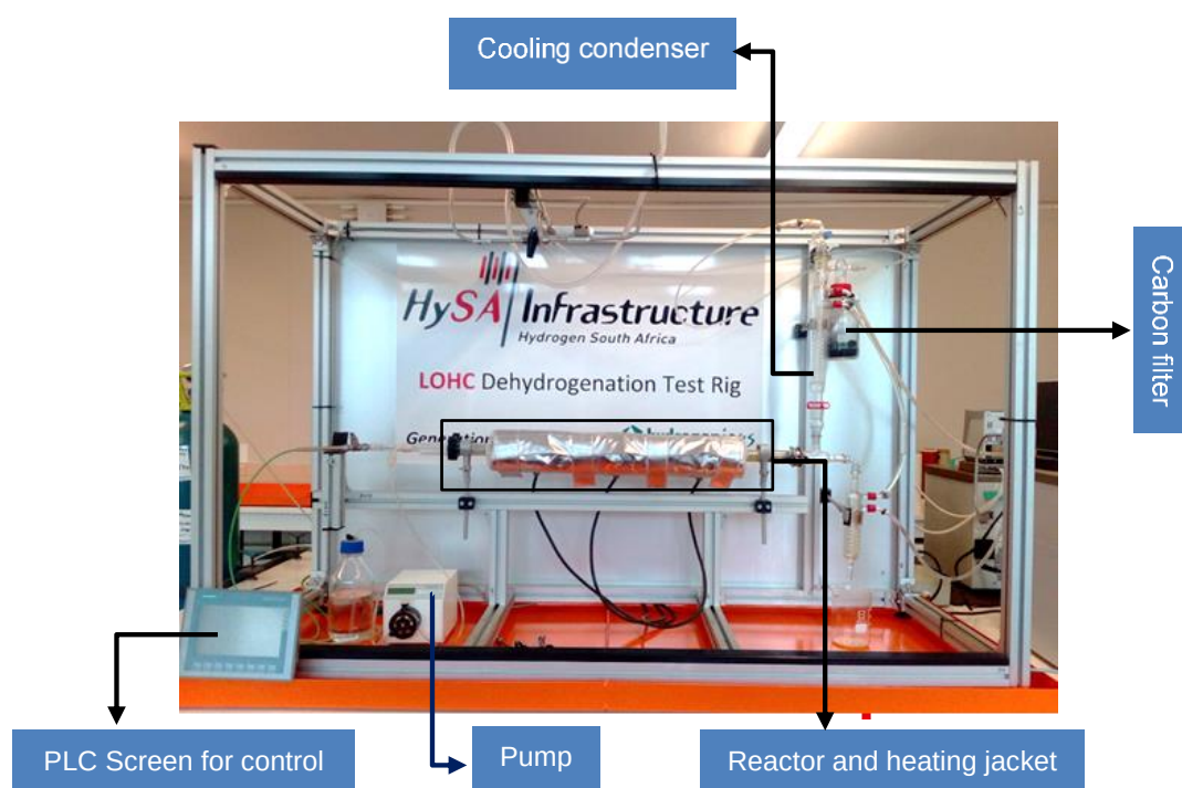
Figure A9: Photograph of LOHC dehydrogenation setup at North West University, supplied by Hydrogenious Technologies GmbH.
