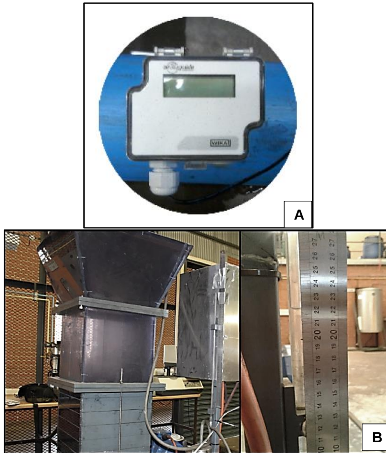
Figure 3.6: Depiction of the flow sensor (A) and water based manometer (B)
