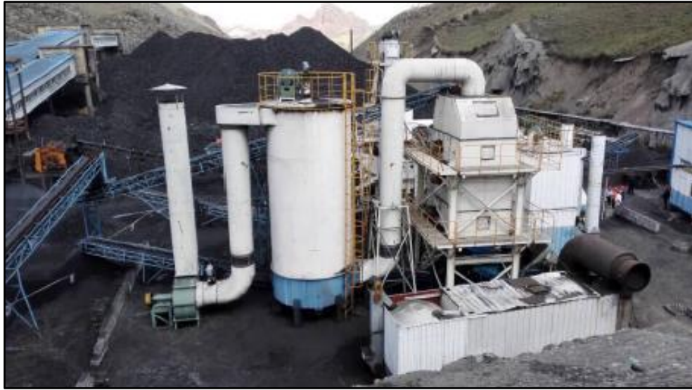
Figure 2.9: Dry dense medium plant in Shenhua, China (taken from de Korte (2016))
