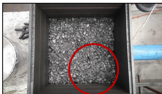
Figure 4.8: Air channelling visible in the bed
