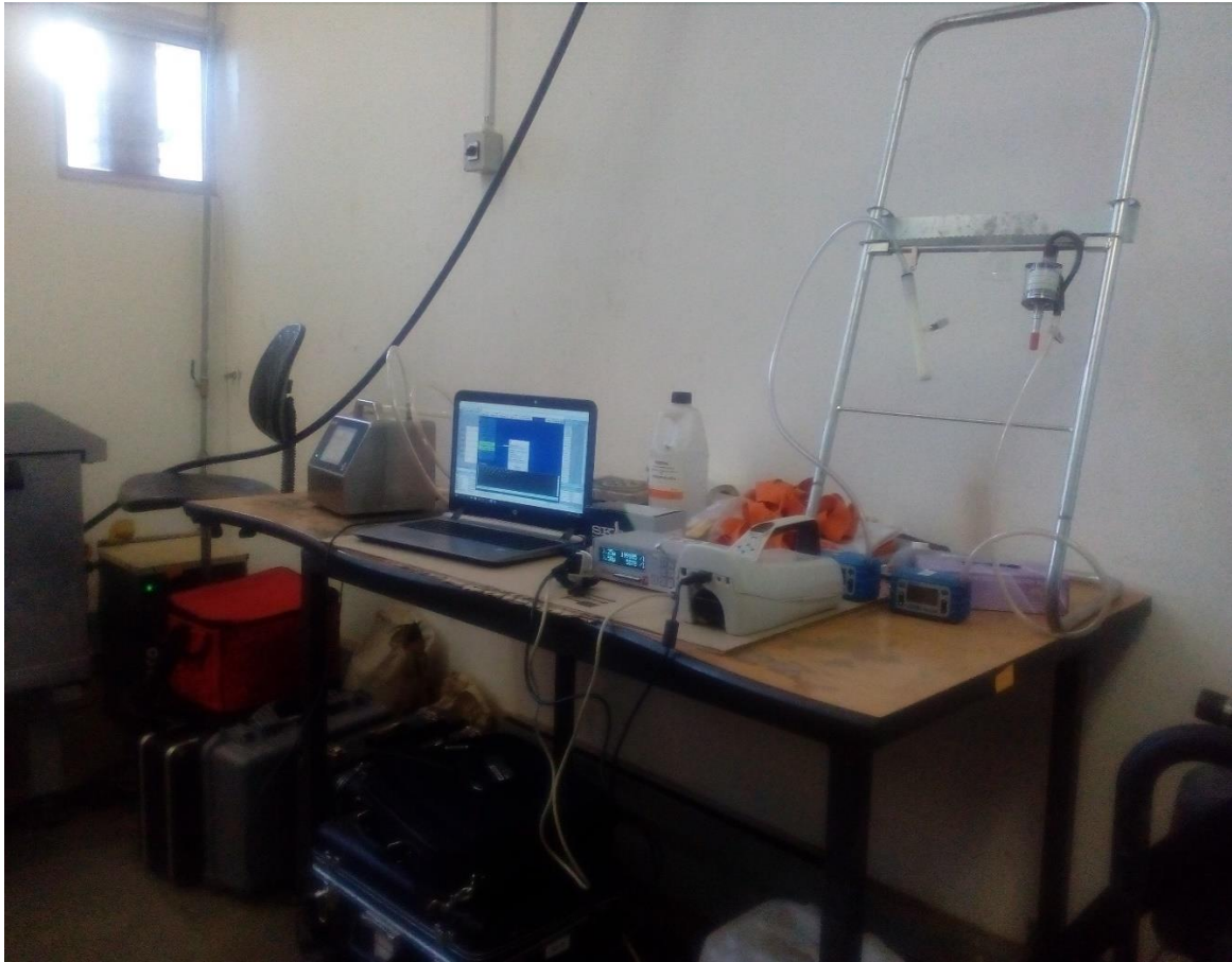
Figure 4-1: Placement of the emission particle sampling instruments on the table 2 m from the AM machine door in the AM machine room at the facility where the study was conducted.
