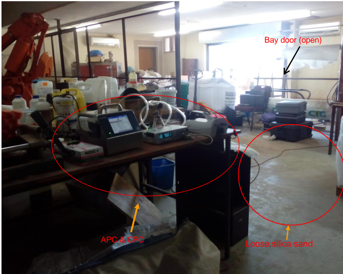
Figure 3-2: An image of the room where the coating process took place showing the bay door being opened as well as the placement of the direct reading instruments: airborne particle counter (APC) APC and condensation particle counter (CPC).
