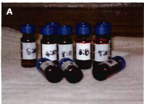
Figure D.9: A) HPLC vials where samples were placed in for analyses and B) Eppendorf Centrifuge system
