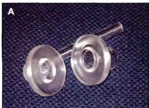
Figure D.6: A) Vertical Franz diffusion cell with donor and receptor compartments and B) Horseshoe clamps
