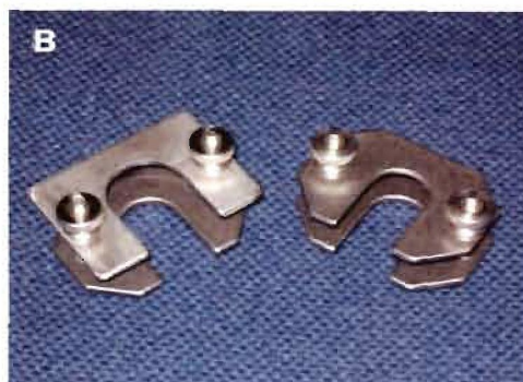
Figure D.6: A) Vertical Franz diffusion cell with donor and receptor compartments and B) Horseshoe clamps
