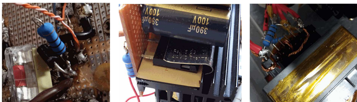
Figure 5-31: RC snubber circuits
