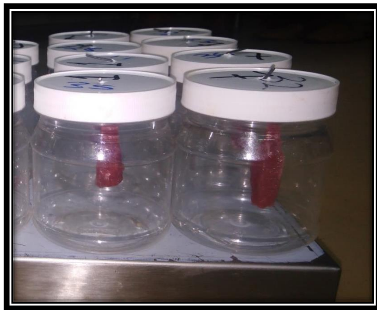
Figure 6. 3 Gravimetric method for measuring drip loss by vertical suspension of meat strips
