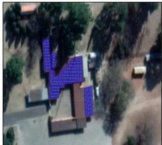
Zuikerbosch Risk 36.5 kWp
