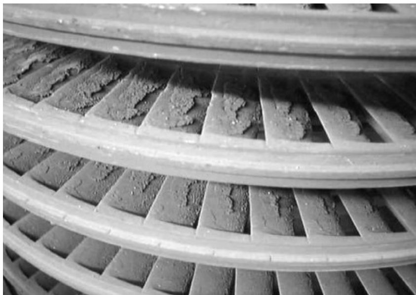
Figure 5.1: Solid particle erosion on a turbine blade [4]
